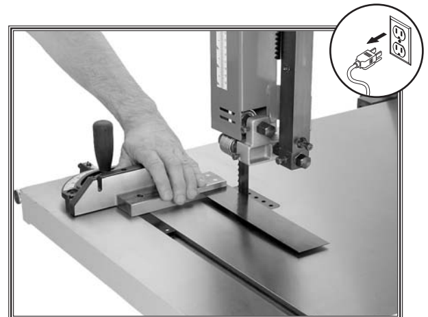
Figure 23. Aligning the miter gauge body with the blade.
